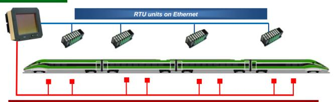
MVBbus: brakes, radio, power line, engine control, power electronics, doors, cockpit, diagnostics, etc.
