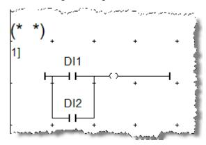
• Double click the coil at the top of the diagram. The following window will appear, which allows you to select a register (also known as a "variable" in ISaGRAF) to be associated with the contact. Select DO5 and click okay:
