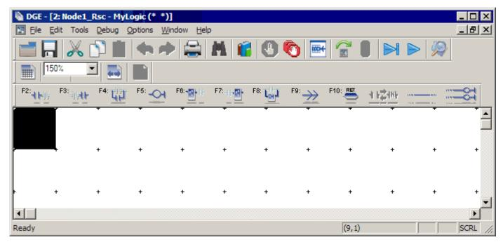
• Click on the button (or press F2) to tell ISaGRAF that you would like to place a contact. Select DI1 as your first register assigned to the contact. The window will then look like this:
