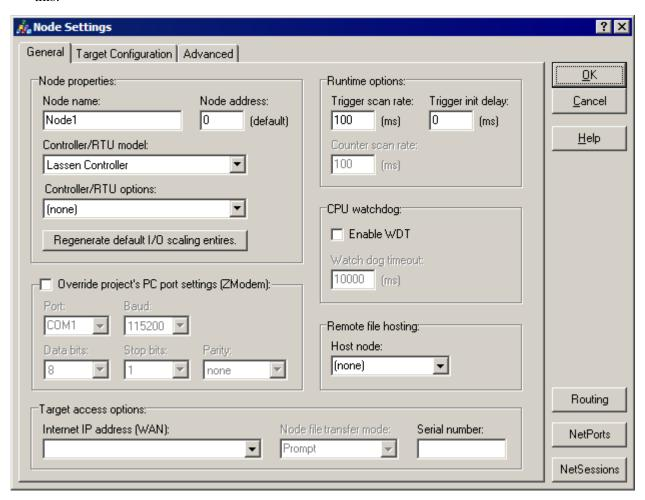
This is your **Node | Settings** window. All controller configuration for debugging, IP configuration, servers and communication options are done here. There are a few basic configurations that we need for a Pinnacle controller such as the Lassen to ease the application development cycle. We need to configure an IP address (mandatory), configure ISaGRAF v5 for debugging over Ethernet and enable the FTP server on the controller.
