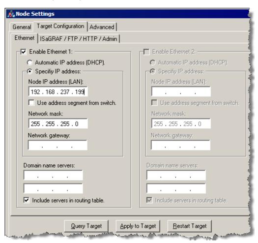
Check the Enable Ethernet 1 and put in a Node IP address (LAN) that is compatible to your network. If you don't know what is compatible, ask your IT person what would be a good address to use for your computer to talk to this controller. If you are connecting straight to the Ethernet port on your computer, the above address will work fine. You will be asked to change the IP on your computer to a compatible address when we attempt to download.
