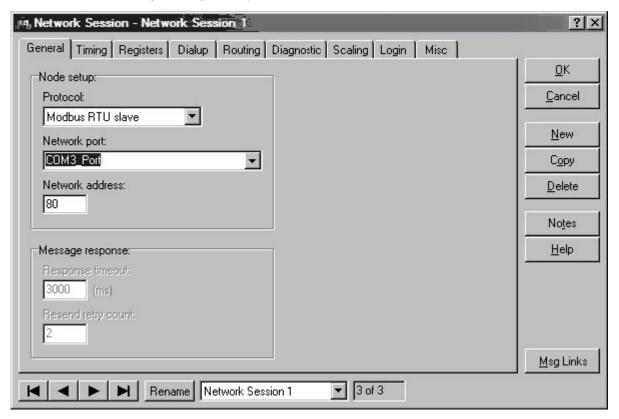
The "Network Address" is used to unique identify the slave. When the master has a message to send to the slave, it uses this address.
