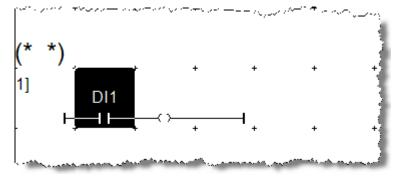
• Notice that the Quick LD editor automatically makes a complete "rung," including a coil.
