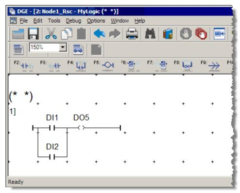
• We are using DI1 and DI2 for simplicity. On Pinnacle controllers, DO5 is a common point to all the controller types but is a slightly different piece of hardware on the Lassen
