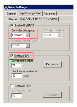
Then Enable ISaGRAF checkbox should already be checked. Set the Controller debug port to "Ethernet".
